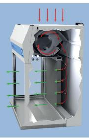
Laminar air flow can be described as an entire body of air flow with steady, uniform velocity.
